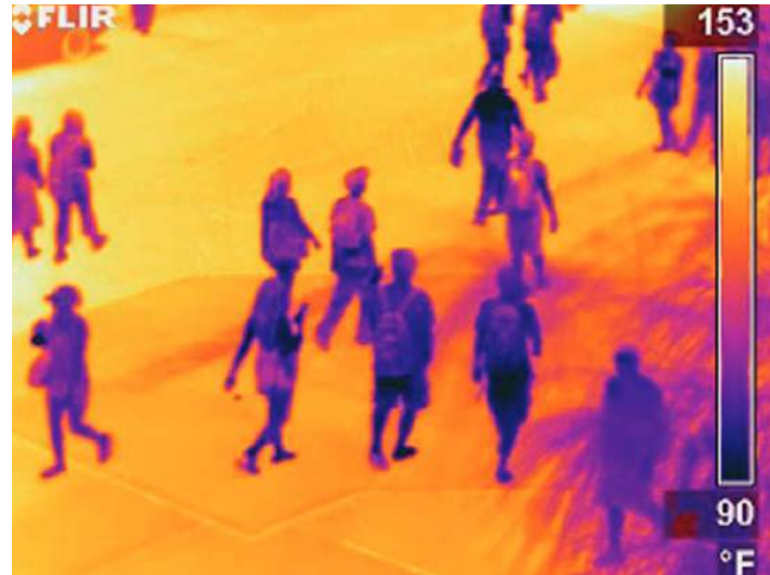
Figure 2.29 - Illustration of the Heat Island Effect of pavement. The color ramp on the right shows the temperatures that correspond to the different temperatures.
