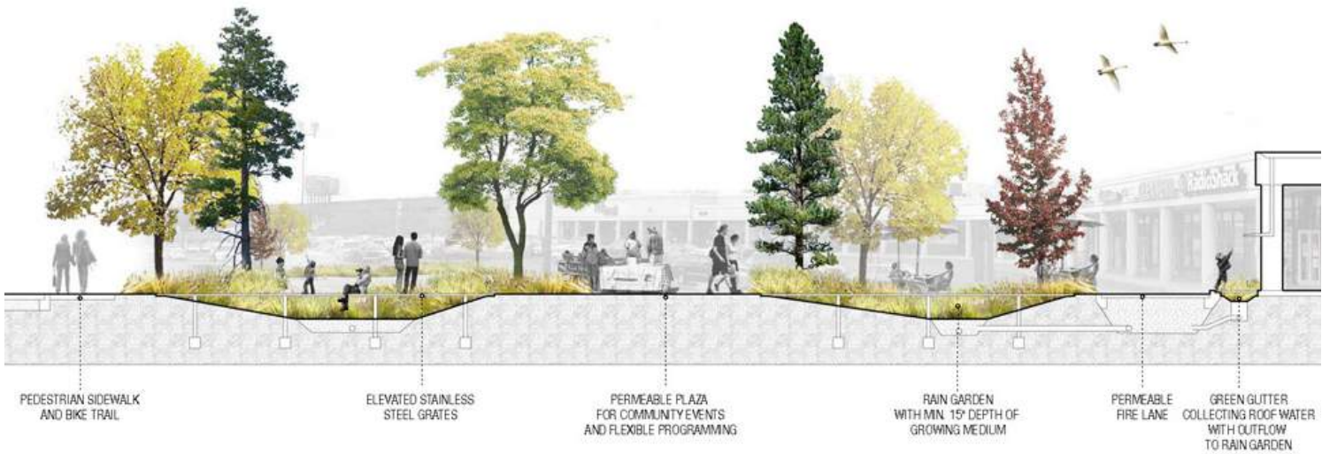
Figure 2.50 - Example of approaches to reduce peak water volumes and increases infiltration.
